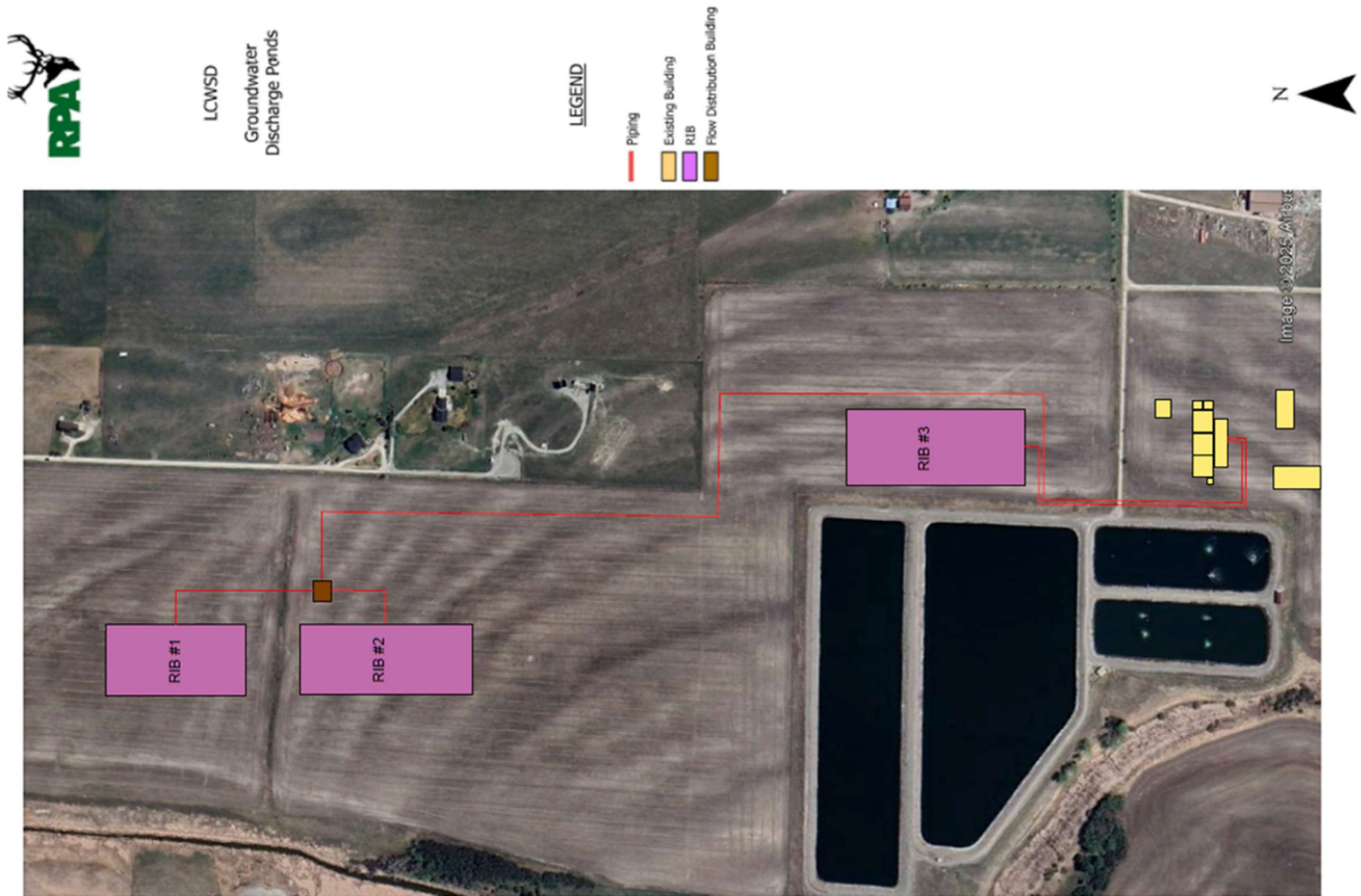
Figure 3. Phase 2 Wastewater Improvements Layout – RIB Locations
